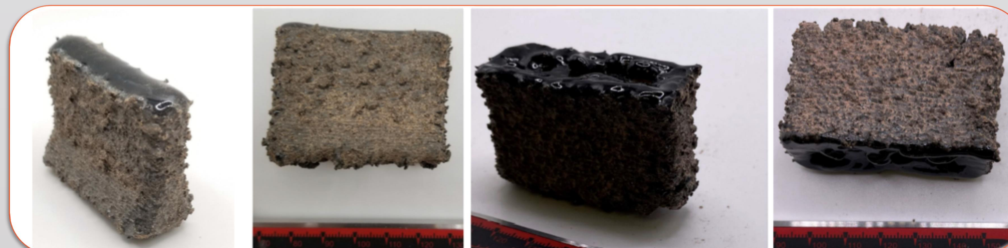
Grousers produced by Outward Technologies SAM system , showcasing different print orientations, the Glass Top grouser (left), and Glass Dove grouser (right). Provided photo is the property of Outward Technologies.
