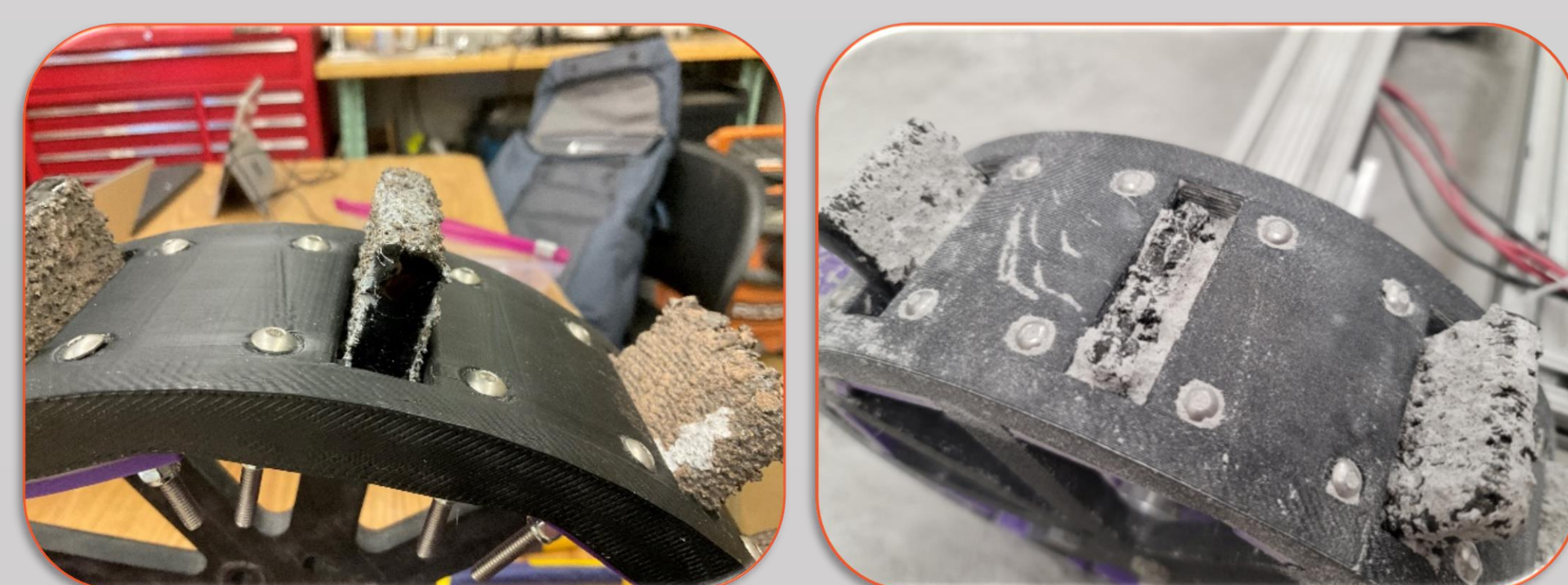
Modular wheels, designed to test different grouser geometries. Regolith parts pictured were produced by Outward Technologies SAM system . Undamaged grousers (left) were installed prior to testing, with damaged grousers (right) inspected once testing was complete.
